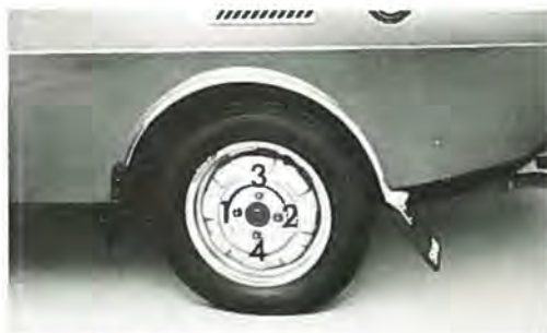
Order of tightening wheel nuts
