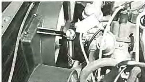
Location of dipstick, automatic transmission
