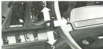
Combined headlight dimmer and flasher switch and direction indicator lever 1. High and low beam, headlight flasher. 2. Left direction indicator. 3. Right direction indicator.
