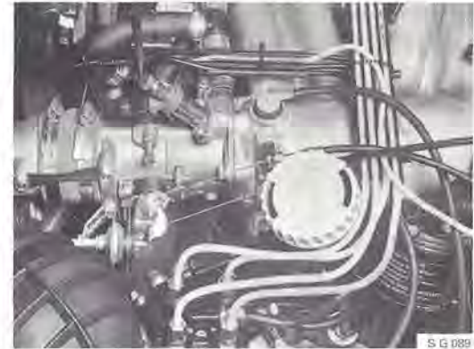
Oil filler cap with dipstick
