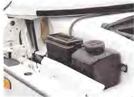
Power steering reservoir
