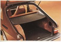
The WagonBack regular large luggage compartment has a capacity of 11½ cubic feet (measured according to SAE standards). An additional space under a covering far back in the luggage compartment adds a maximum volume of 3 cubic feet so even with the rearwindow shelf left in you still have more luggage space than most other cars in our class.
