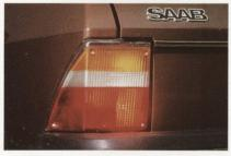
The tail lights have been designed to be clearly visible, even from the sides. The back-up lights direct their beams both backward and downward to make backing up easier and safer at night. The license plate light, incidentally, is built into the tailgate handle.
