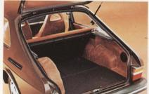
The removable shelf is mounted on two tracks — one on each side — and can be easily and quickly taken out. At the rear of the backrest, flush with the shelf, is a beam that conceals the lock mechanism for the seat backrest. It also functions as a point of attachment for special removable headrests (optional).
