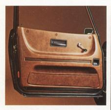
The door panels in the Wagon-Back are of the same type as those used in the Saab EMS: moulded in one piece of impactabsorbing material. Together with built-in, sturdy door beams, our new door panels offer excellent side impact protection.
