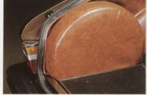
The luggage space has been designed for both function and elegance. The flat floor is covered entirely with vinyl reinforced textile carpeting. And the sides, like the insides of the front doors, are panelled with impact-absorbing materials covered with sturdy vinyl.
